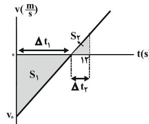
$$\left. \begin{aligned} S_1 + S_2 &= 20m \\ -S_1 + S_2 &= -10m \end{aligned} \right\} \Rightarrow \begin{cases} S_1 = 20m \\ S_2 = 10m \end{cases}$$
